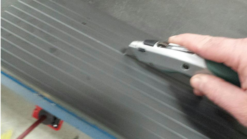
**TIP:** Score the underside of the metal 10 times with a new blade (sharp). Grasp the metal on each side of the score and bend the metal back and forth to get it to break at your cut.
