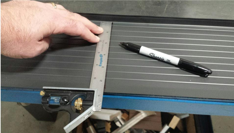
**TIP:** It is important to make a 90 degree cut. Take your time and use the snips to cut along your mark. Cut from each side towards the bend.
