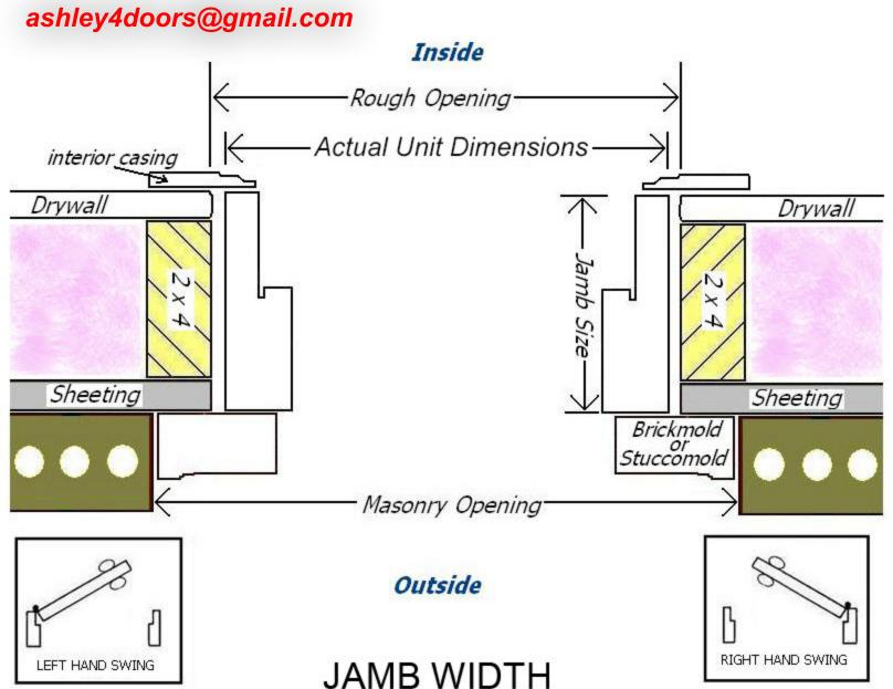
To measure the width of the jamb, open the door and measure the jamb, Do not include any of the trim work or casing or brickmolding.
